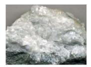
Magnesite is the blue stone Satka is famous for. In reality it is primarily grey in color. It is used to produce refractories, they are materials that can withstand extremely-high temperatures. Magnesite products are mainly used in metallurgical factories for iron production, but their scopes of application also include non-ferrous metallurgy, cement, chemical, pulp and paper industries, energy, and agriculture.
